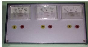
Insulation-Meter. For testing components tubes, diodes, capacitors, resistors.....
