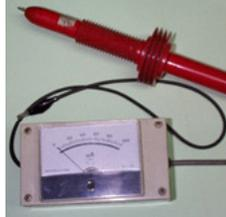
Grid Current Galvanometer. To measure an tune grid current. Drawing with electronic components to improve the measurements.
